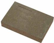
**BetonWood N** The BetonWood N cement bonded particle boards, with high density (1350 Kg/m<sup>3</sup>), made of Portland-type cement conglomerate and debarked Pine wood fiber. These panels have the following thermo-dynamics characteristics: thermal conductivity coefficient  $\lambda=0,26$  W/mK, specific heat  $c=1,88$  KJ/Kg K, coefficient of resistance to vapor penetration  $\mu=22,6$  and reaction to fire class A2-fl-s1, according to the standard EN 13501-1.
