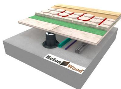
Complete dry system for elevated floors with Betonradiant radiant panels, wood fiber Underfloor panels and BetonWood TG cement bonded particle boards on adjustable supports. Excellent construction system for floating radiant floors.
