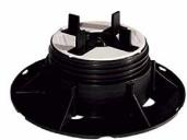
**Adjustable supports SB** Adjustable Floor Stands have anti-noise rubber head, specific adjustment key, variable heights, pre-cut base for wall corner cutting. Possibility to adjust the height millimetrically (adjustable from 25 to 270 mm), in favor of a perfect leveling of the flooring.
